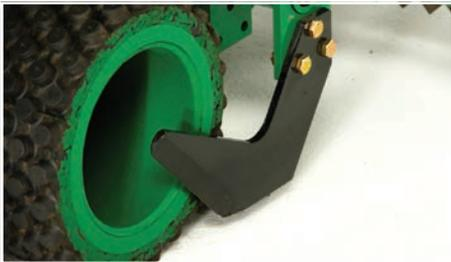
Durable cutting blade is easily adjustable down to a depth of 2 1/2" and can change angles to match soil and blade conditions.
