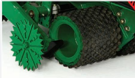
A forward metering wheel helps measure and cut sod accurately.
