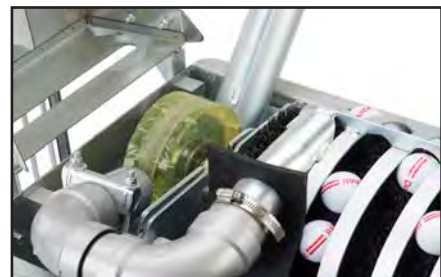
After washing the composite loader wheel pushes the balls into the feeder pipe.
